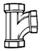
Hub x hub x hub. Used to connect vertical branch line into straight sewer line. Also, used with cleanout to provide access to piping.
