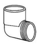
Slip x MIP. Used to change direction in piping. Adapts to standard female pipe threads. Teflon joint tape is recommended for threaded joints.
