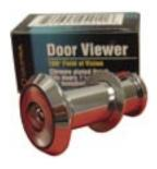
One-way viewer is zinc die-cast with 180° angle plastic lens. 9/16" diameter, adjusts for door thicknesses 1-1/2" to 2-1/2". Installation hole is 9/16". Display boxed.
